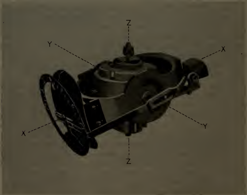
FIGURE 31.—Gyro horizon mechanism in climb.
